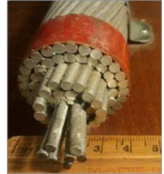
An aluminium conductor steel-reinforced cable (ACSR) cable, the steel strands are in the middle.
