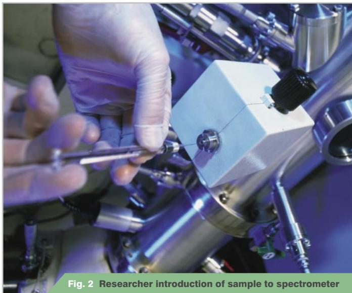
Fig. 2 Researcher introduction of sample to spectrometer
