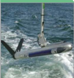
In this technique a torpedo-shaped device called a *towfish* (Fig. 4) is towed through the water close to the seabed at a speed of about 2 km/h. The towfish contains *ultrasonic transducers* and underwater microphones (hydrophones). Very high frequency ultrasound pulses (typically 100 kHz to 500 kHz) are directed laterally and the echoes are picked up by the hydrophones. The resulting data is processed to produce images of extraordinary resolution (down to a few centimetres).
